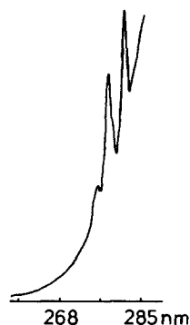
FIG. 3. The {}^6I \rightarrow {}^8S line emission of \text{Gd}^{3+} in \text{YTaO}_4:\text{Gd} at the onset of the tantalate emission band.
